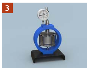
Tests to define resistance to sulfide stress-corrosion cracking
