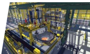
TWIN TANK VACUUM DEGASSER
